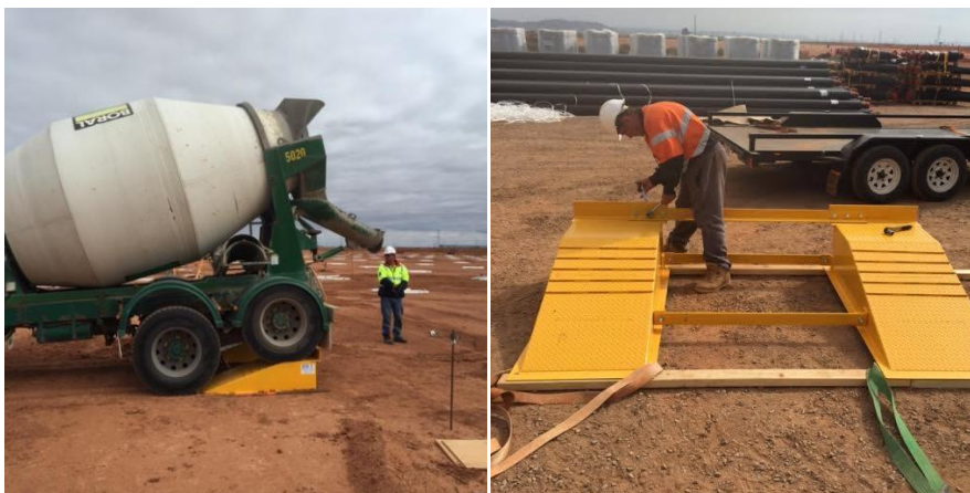
Above photographs: Rated ramps designed and built by BRT
