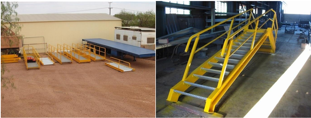
Above Photographs: Wash-down platform designed in segments for easy transport
